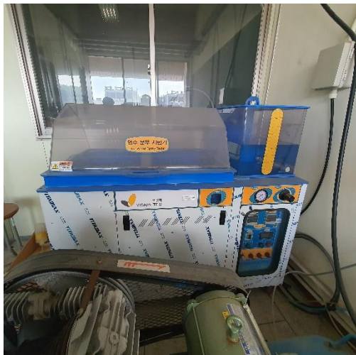
Salt spray corrosion test
